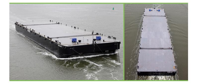
The Tobias is a heavily constructed modern flat deck project barge. It has an intergrated ballast system and is capable of ballasting to her LL depth. A reliable and versatile unit, the Tobias serves the Project / Transportation fleet.
