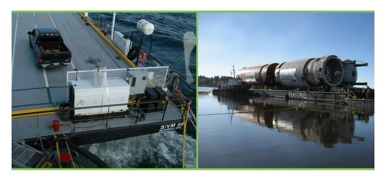
Special features include, steel deck construction and moveable spud wells. Ideally suited for use as a construction platform, it also transports cargoes. A reliable and versatile unit, the S/VM 86 services the Project fleet.
