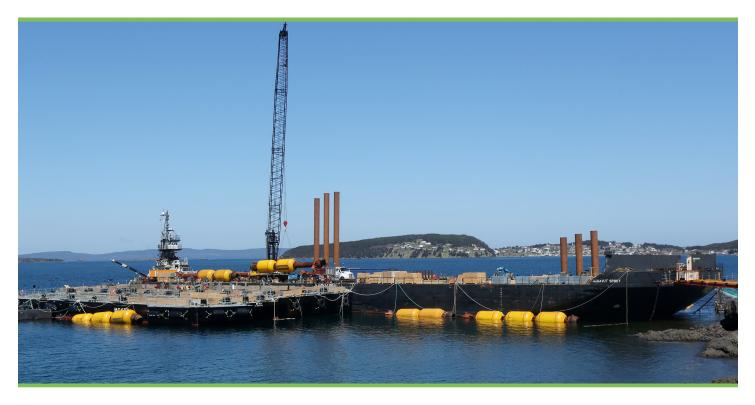
A dual purpose 12,000 tonne docking and flat deck barge. Special features include capability to be rigidly secured on 6 X 4' dia. spuds in over 30m depth of water. It is Ocean classed. A reliable and versatile unit, the Nunavut Spirit serves the Project & Transportation fleet.
