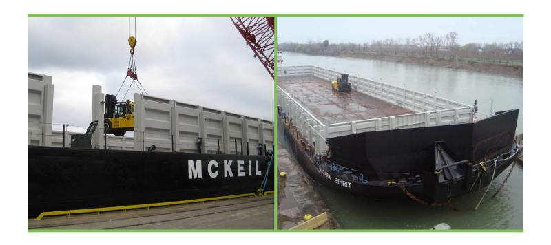
Special features of this flat deck cargo barge include removeable bin wall access points for side loading and a steel deck for customized lashing configurations. This barge is capable of being ballasted and is a versatile unit serving customers in a range of dry bulk commodities and cargo sectors.
