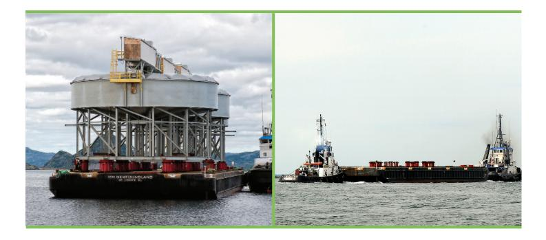
The MM Newfoundland is a flat deck multipurpose barge. Special features include a steel deck with 4,500 lbs per square foot deck strength, making it the strongest deck barge in Eastern Canada. A reliable and versatile unit, the MM Newfoundland services the Project / Transportation fleet.
