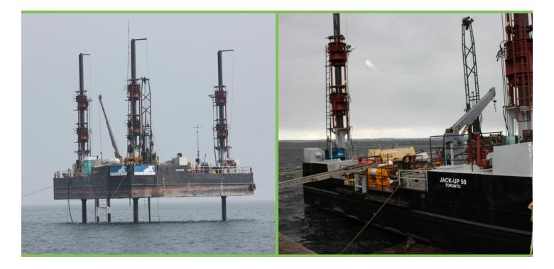
The Jack Up 50 is a versatile asset supporting the project fleet. Features include a deck load capacity of 45 tons when in tow and a lifting capacity of 15 tons up to 100'. The barge is ideally suited for use as a platform for drilling or other construction projects.
