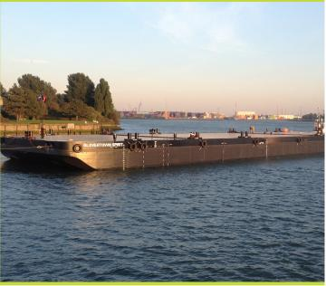
The Glovertown Spirit is a heavily constructed modern flat deck barge. Special features include a steel deck with 20 tonne per square meter deck strength. A reliable and versatile unit, the Glovertown Spirit services the Project / Transportation fleet.
